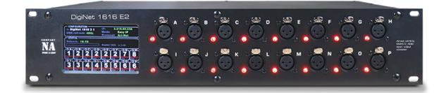
16-way Bidirectional ArtNet/sACN-DMX Node with RDM support. Device has Dual EtherCon Ports and PoE Power in, sixteen DMX ports, which are galvanically isolated and can be configured as inputs/outputs. Configuration of the node can be done using built-in web server or DigiNet Manager. Gigabit Ethernet allows for this unit to be used in large networks without affecting performance. Large TFT touchscreen allows for quick setup and easy maintenence.
