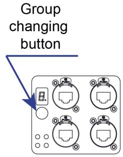
To change port group, hold button for few seconds to unlock group, then press of the button will cycle trough all available groups (visible on the seven segment display). After required group is selected, wait for a few seconds for this new group to be saved and for switch to reconfigure ports.
